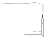
Place the textile print in the frame. Start with the corners and press the silicone strip in the channel.
