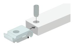
Put the stabilizer on the lockset, now tighten the screw with the delivered allen key.
